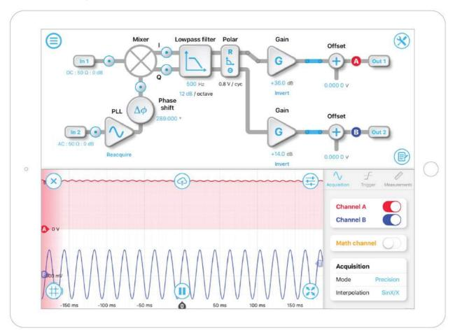
8. Tune the gain values in each arm to balance precision and measurement range.
