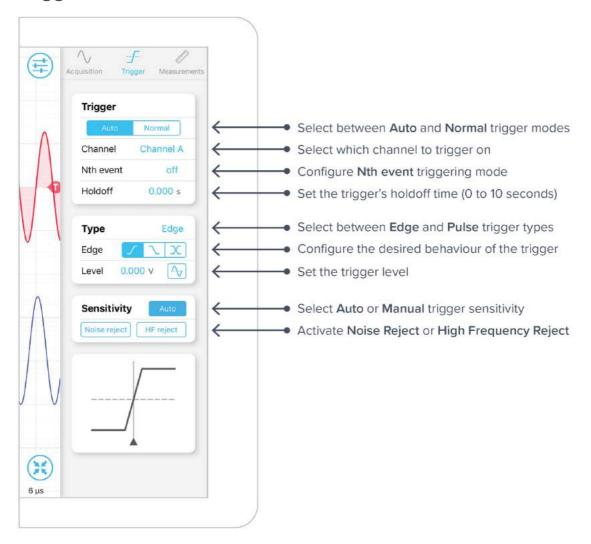
**Tip:** Quickly adjust trigger settings by tapping the trigger marker  $\mathbf{q}$
