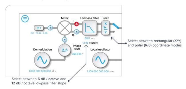
Rectangular (or Cartesian) coordinate mode measures the input signal with respect to a specific quadrature of the reference signal. When combined with a PID controller, Cartesian mode can be used to perform laser frequency stabilization.
