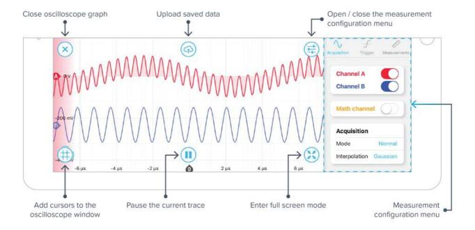
The oscilloscope will appear automatically when a probe point
