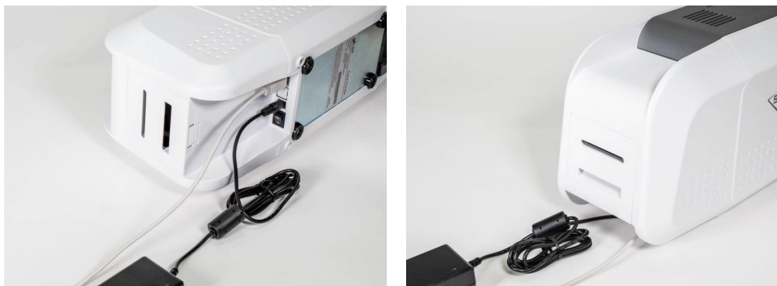
Figure 10 SMART-51D Connection of power and USB cable
