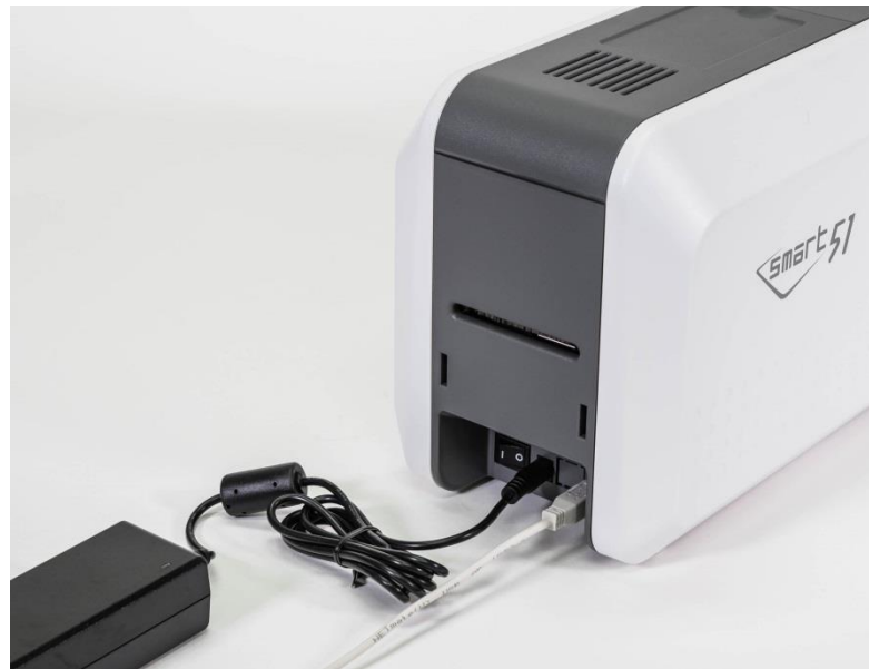
Figure 9 SMART-51S Connection of power and USB cable
