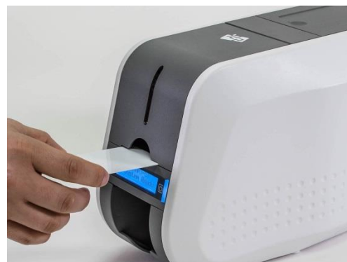
Figure 29 Loading the cards 3
