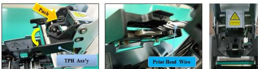
Figure 114 Print head replacement
